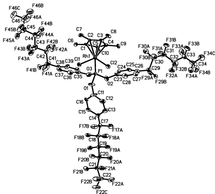
**Figure 1.** Molecular Structure of  $[\text{Cp}^*\text{RhCl}_2\{\text{P}(\text{OC}_6\text{H}_4-4-\text{C}_6\text{F}_{13})_3\}]$  (**9c**). Displacement ellipsoids are shown at the 30% probability level. The H atoms are omitted for clarity.
